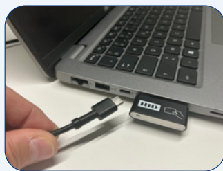
USB-C connector on the edge to keep other ports available when the readers are in use.
